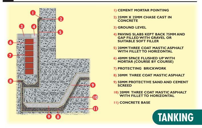
Externally applied mastic asphalt tanking over pile caps or under column bases
