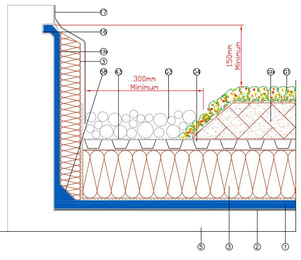
I-20MM TWO COAT MASTIC ASPHALT
